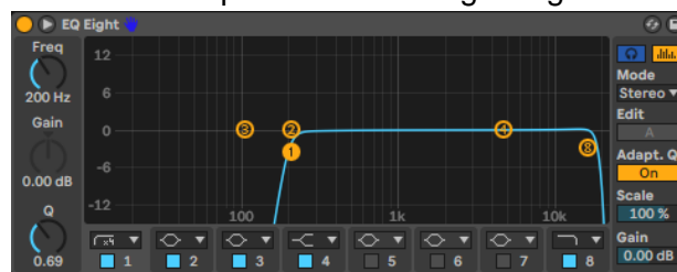
Figure 1.7 EQ to remove low end thump and noise
