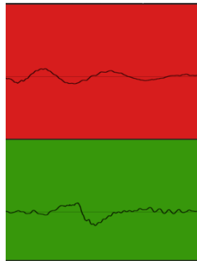
Figure 1.4 Bass DI out of phase with Bass Amp
