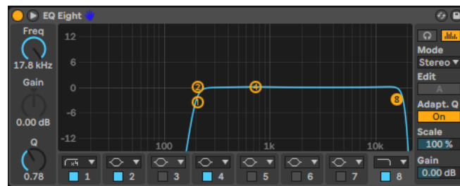
Figure 2.4 High Pass Filter on Duplicated Bass Track
